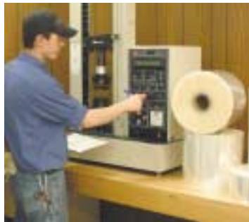
Lab manager Rob Teschke checking the finished rolls of film for tensile strength, gauge, gloss and co-efficient of friction.
